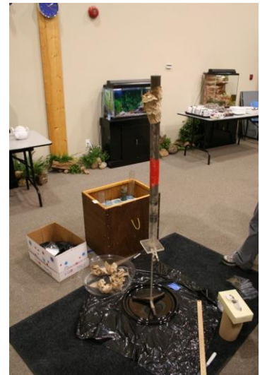
The core is sectioned into discrete intervals by pushing the sediments up from the bottom of the core tube and removing the sediments from the surface of the core.
