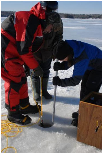
The corer and core tube are lowered through the ice and the core tube is manually pushed into the sediments to the desired depth using the push rod.
