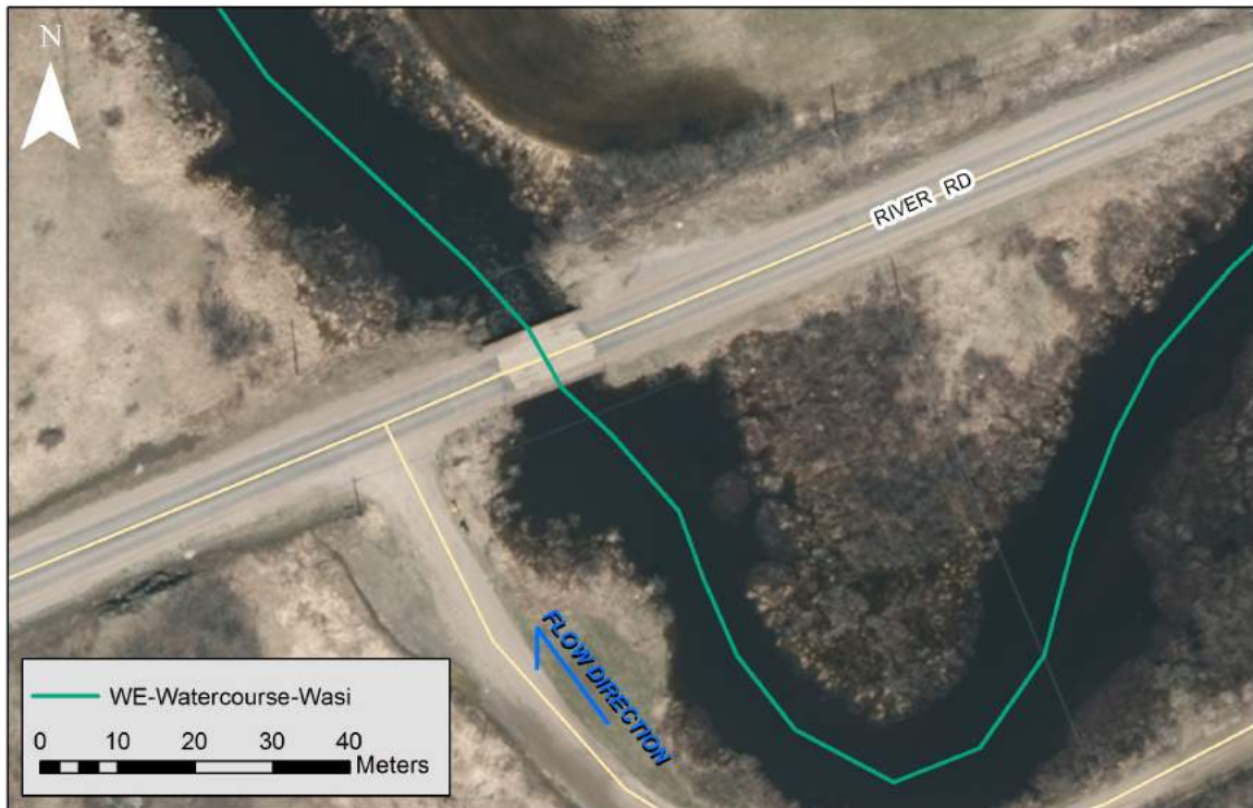
Figure 2.10: Undersized crossing span relative to channel geometry.
