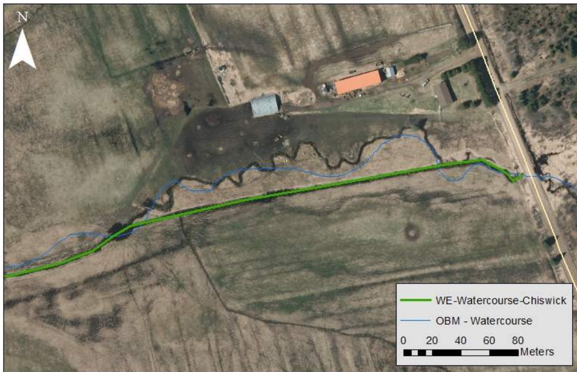
Figure 2.8: Channelization along Chiswick Creek.
