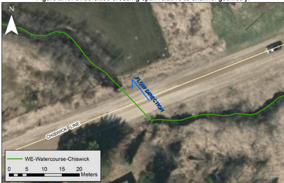
Figure 2.11: Undersized crossing span, and inappropriate skew. Tight bend at culvert inlet.
